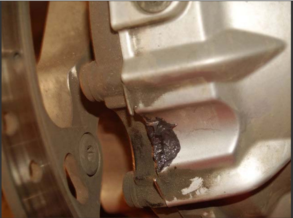
A close-up of the notch shows how we added a little grease to protect the FD paint. (Turning down the Torx even further will eliminate the need for that!)
